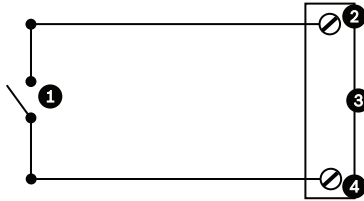
Figure 6.3 N.O. - Normally Open Non-supervised Connections
